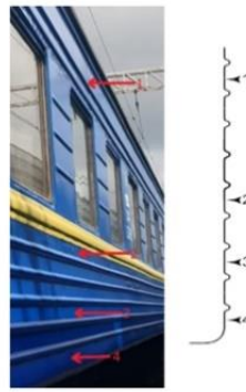
Fig. 5. Scheme of side wall paneling measurements
