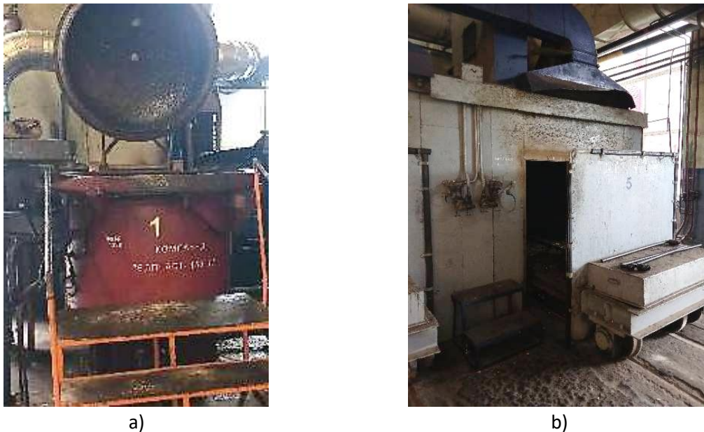
Fig. 3. Autoclave for rotor impregnation (a) and drying oven for drying (b)
