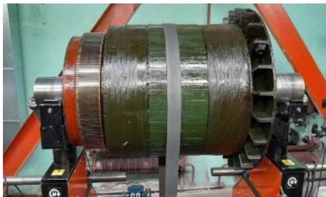
Fig. 2. Balancing machine EI2000 with the rotor of the electric motor 1DT-003 installed for balancing
